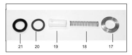
11. Remove the guided p-valve, (19), valve springs (18), v-sleeves (21) and pressure rings (20). Inspect for wear and replace as necessary. Remove the spacer ring (17) from the plungers (8).
