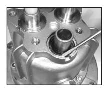
12. If the crankcase oil seals (15) are to be replaced, they can be removed by prying loose with a screwdriver. Take care not to make contact with the plunger (8) and pry out the oil seals from their housing. Seals should not be reinstalled until after step
