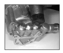
10. Tap the back of the manifold (35) with a rubber mallet to dislodge, and slide off the plungers. (8). Take note of the position of the discharge port so as to place the manifold in the same position during reassembly.
